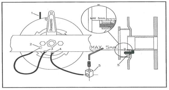
Drawing "B" Attaching cable to wire drum
